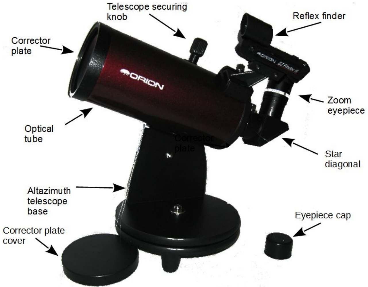
Illustration 1: Telescope Parts - side view
