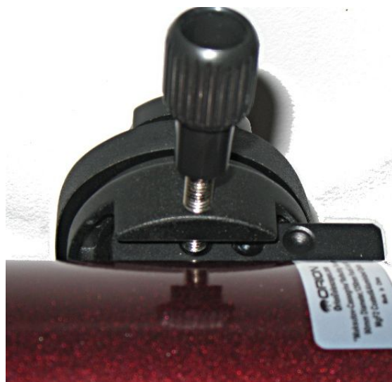
Illustration 4: Telescope securing knob in the forward storage indentation in the Dovetail bar
