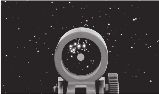
Illustration 6: The EZ Finder II superimposes a tiny red dot on the sky, showing right where the telescope is pointing.
